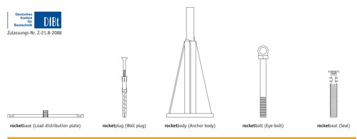
Professional permanent scaffold anchor for ETICS, VCW and Cavity wall. Approved for use on masonry according to DIN 4426 (German standard) with ideal force dissipation. Remains permanently in the façade and can be reused at any time.
